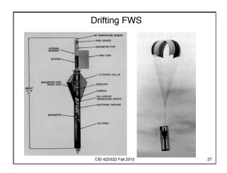
Floating weather stations (FWS) are buoys that float at sea and that are equipped with sensors to monitor weather conditions. Each FWS has an on-board computer that maintains a history of recent weather data. At regular intervals the buoy transmits the weather data using a radio transmitter.
